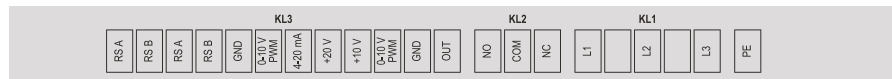
Wiring diagram of the fans: ADNAX PROFI 800x500, ADNAX S PROFI 800x500 ADNAX PROFI 900x500, ADNAX S PROFI 900x500, ADNAX PROFI 1000x500 ADNAX S PROFI 1000x500
